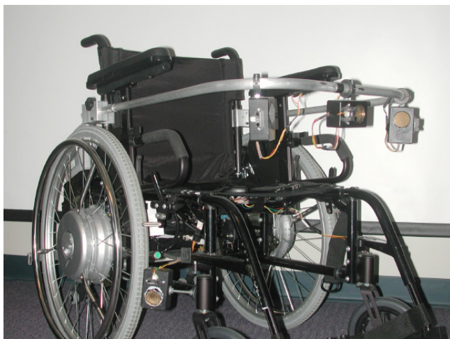
Figure 1 The Smart Power Assistance Module for Manual Wheelchairs (front view).
