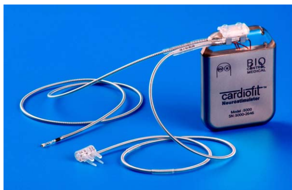
Fig. 4. Image of the CardioFit system, an investigational device aimed at the treatment of congestive heart failure. It consists of a dual-cathode circumneural multi-polar stimulation lead and a sensor lead. The sensor lead is placed in the hearts right ventricle and the stimulation lead wraps around the vagus nerve. The system sends electrical pulses from the stimulator to the vagus nerve, and detects changes in heart activity to modulate the stimulation (Courtesy of BioControl Medical, Yehud, Israel). 40
