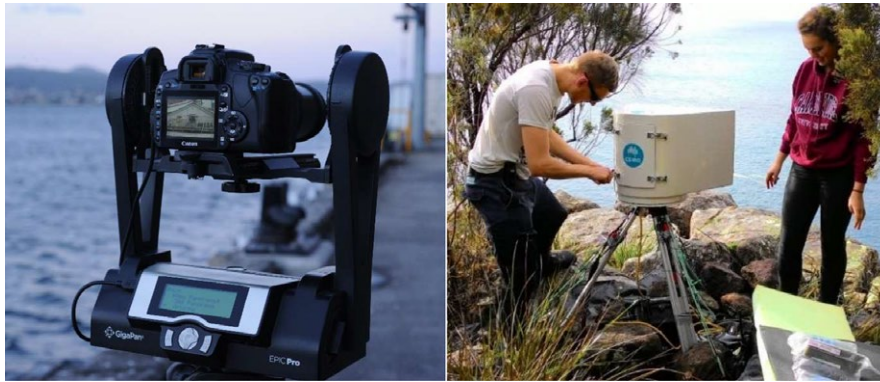
FIGURE 2 An unmodified GigaPan Epic PRO unit (left) and a CRAGS deployed at Waterfall Bay, SE Tasmania (right)
