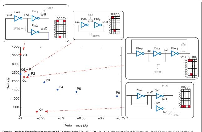
Figure 5 Pareto front for a maximum of 3 active pairs ( $Q_1, Q_2 = P_1, Q_3, Q_4$ ). The Pareto front for a maximum of 2 active pairs is also shown. Blue dots represent circuits with 2 active pairs and red dots represent circuits with 3 active pairs.
