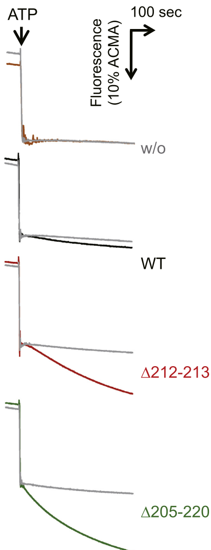
Figure 4. Measurements of the proton-translocating activity of proteoliposomes. The reaction was initiated by the addition of 2 mM ATP to proteoliposomes containing F_0F_1 with (gray) or without 1 \mu\text{g ml}^{-1} FCCP at 30^\circ\text{C} . The inside acidification was monitored with fluorescence quenching of ACMA (excitation at 410 nm, emission at 480 nm). Liposomes were used as the negative control (w/o).
