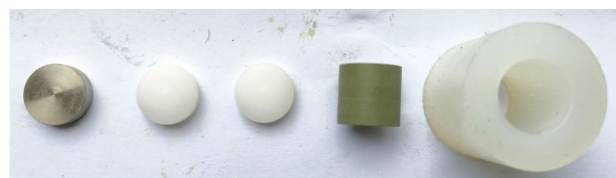
(a) Photographs of the steel sheet, upper PE, lower PE, explosive sample, and soft confinement before the impact test.
