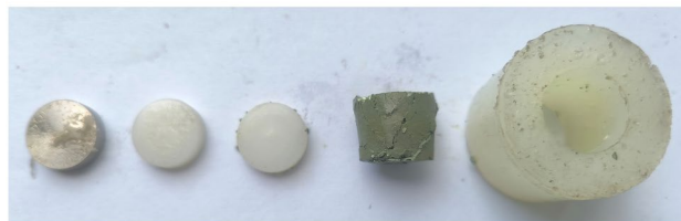
(b) No reaction, photographs of the steel sheet, upper PE, lower PE, explosive sample, and soft confinement after the impact test.
