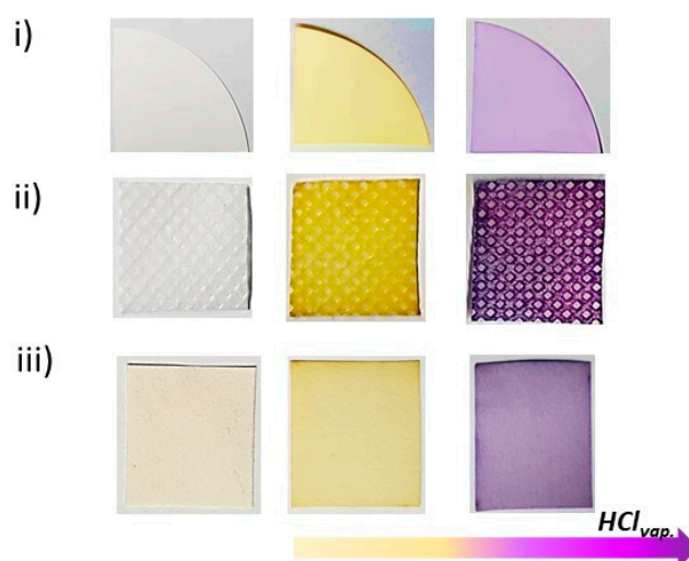
Figure 6. Nylon (i), cotton (ii), and filter paper (iii) dyed by dipping into a 5 mM methanol solution of cyanine 1. Rows (i)–(iii): Left: before dyeing, middle: dyeing with 1; right: after exposure to acidic vapors.
