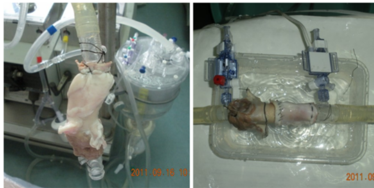
Figure 3 The static and releasing tests of aortic valved stent in PVC tube.
