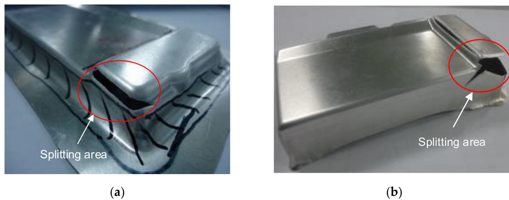
Figure 18. The experimental forming results for Case I. (a) The first stage; (b) the second stage.
