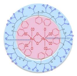
**Figure 11.** SMA/CORM2 micelle structure. In blue SMA formed a hydrophilic outer surface, in red CORM2 formed a hydrophobic core [76].
