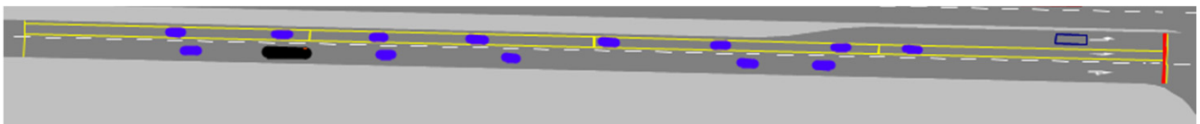
Figure 3. Graphical representation of the roadway in Vissim split into four parts on one lane ( n_1 = 1 , n_2 = 5 , n_3 = 4 , n_4 = 3 ).
