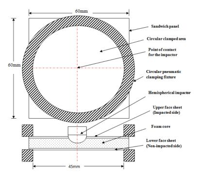
**Figure 3.** Line diagram illustrating pneumatic circular clamp dimensions of the drop weight impact test machine with the specimen [52].
