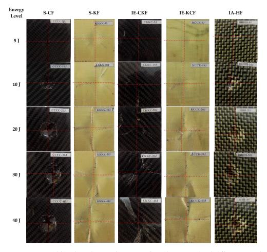
Figure 6. Impacted face sheet photographic images of samples impacted with different energy levels.
