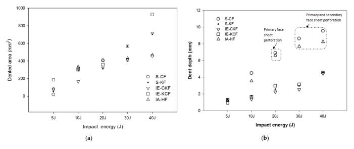
**Figure 33.** (a) Dented area on the top facing sheet of various sandwich panels. (b) Dent depth of the top facing sheet of sandwich panels with respect to the different energy levels.
