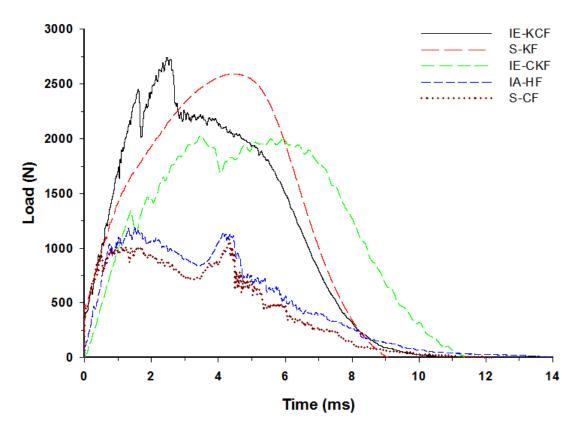
Figure 14. Load-time history of different foam core sandwich specimens at 20 J.
