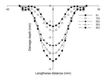
**Figure 29.** Residual dent depth with respect to the lengthwise distance of  $[K_2/Foam \text{ core}/K_2]$  sandwich specimens impacted with different energy levels.
