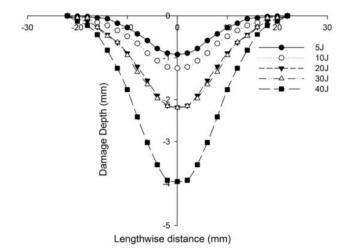
**Figure 30.** Residual dent depth with respect to the lengthwise distance of [C/K/Foam core/K/C] sandwich specimens impacted with different energy levels.
