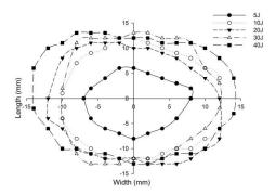
**Figure 26.** Graph illustrating incident face sheet damage area of [H<sub>2</sub>/Foam core/H<sub>2</sub>] sandwich specimens corresponding to different impact energy levels.
