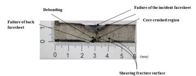
**Figure 5.** Photographic example of through-the-depth local indentation of the foam core sandwich panel under low-velocity impact after the three stages of the penetration progression: (i) failure of incident face sheet, (ii) core crushing and shearing failure, (iii) failure of the back face sheet.
