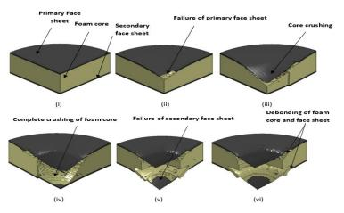
**Figure 35.** The progression of damage to the face sheet and foam core at various stages of impact (i) before the impactor contacting the primary face sheet (ii) failure of primary face sheet (iii) core crushing (iv) complete crushing of the core (v) failure of the secondary face sheet (vi) debonding of foam.
