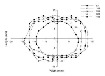
**Figure 22.** Graph illustrating incident face sheet damage area of  $[C_2/Foam \text{ core}/C_2]$  sandwich specimens corresponding to different impact energy levels.
