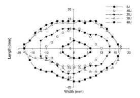
**Figure 24.** Graph illustrating incident face sheet damage area of [C/K/Foam core/K/C] sandwich specimens corresponding to different impact energy levels.
