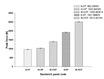
Figure 18. Comparison of peak force of different foam core sandwich specimens at 10 J.
