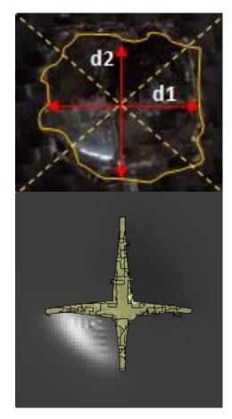
**Figure 27.** Photograph illustrating the measurement of length of the surface damage d1 and d2 on incident (primary) face sheet of  $[C_2/Foam \operatorname{core}/C_2]$  with the numerical simulation result.
