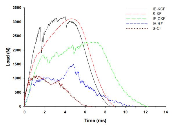
Figure 15. Load-time history of different foam core sandwich specimens at 30 J.
