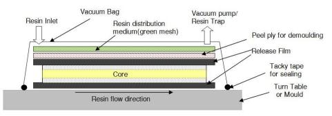
**Figure 1.** Graphic representation of Vacuum-Assisted Resin Transfer Molding (VARTM) fabrication process for foam core sandwich panel.
