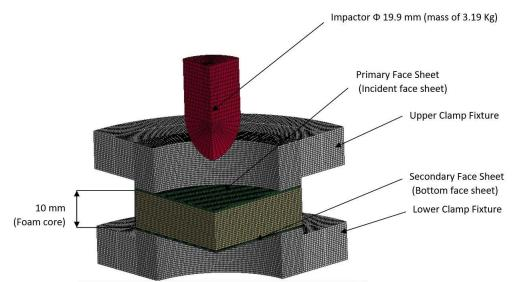
Figure 11. The FE model of foam core sandwich panel with the circular clamp fixture and impactor.
