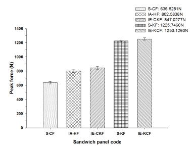
Figure 17. Comparison of peak force of different foam core sandwich specimens at 5 J.
