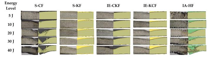
**Figure 34.** Comparison of experimental and numerical failure modes of sandwich panels subjected to varying levels of impact energy.
