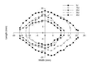
**Figure 23.** Graph illustrating incident face sheet damage area of  $[K_2/Foam \text{ core}/K_2]$  sandwich specimens corresponding to different impact energy levels.
