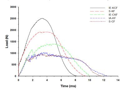
Figure 13. Load-time history of different foam core sandwich specimens at 10 J.
