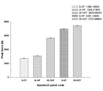
Figure 21. Comparison of peak force of different foam core sandwich specimens at 40 J.
