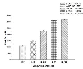
Figure 20. Comparison of peak force of different foam core sandwich specimens at 30 J.
