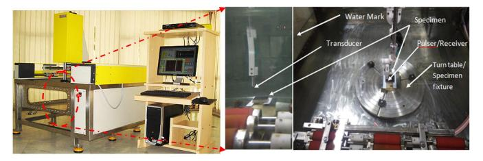
**Figure 10.** Ultrasonic immersion C-Scan testing system showing the water immersion tank with specimen turn table.
