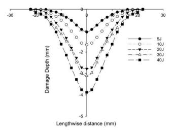
**Figure 31.** Residual dent depth with respect to the lengthwise distance of [K/C/Foam core/C/K] sandwich specimens impacted with different energy levels.
