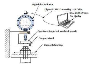
**Figure 9.** Line diagram depicting the process of determining the incident face sheet residual depth high-precision micrometer gauge after impact.
