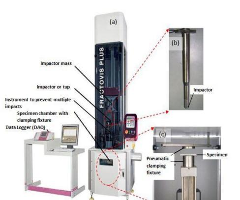
**Figure 2.** Low-velocity drop weight impact test machine with the data acquisition system (DAQ) and clamping fixture. (a) Drop weight machine. (b) Impactor of 19.9 mm diameter. (c) Pneumatic clamping fixture.
