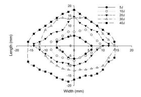
**Figure 25.** Graph illustrating incident face sheet damage area of [K/C/Foam core/C/K] sandwich specimens corresponding to different impact energy levels.
