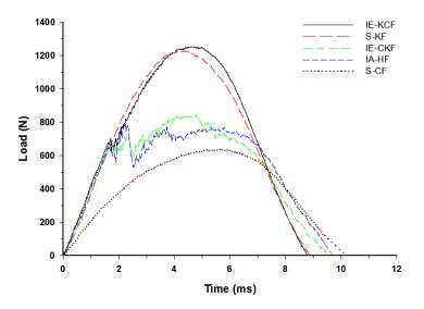
Figure 12. Load-time history of different foam core sandwich specimens at 5 J.
