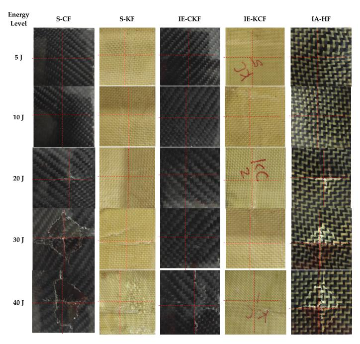
Figure 7. Secondary face sheet photographic images of samples impacted with different energy levels.
