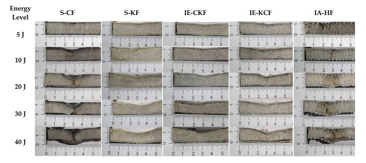
**Figure 8.** Transverse damage morphology of various foam core sandwich specimens after impact with hemispherical impactor shows the residual indentation, delamination, debonding, core crushing.
