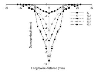
**Figure 28.** Residual dent depth with respect to the lengthwise distance of  $[C_2/Foam \text{ core}/C_2]$  sandwich specimens impacted with different energy levels.
