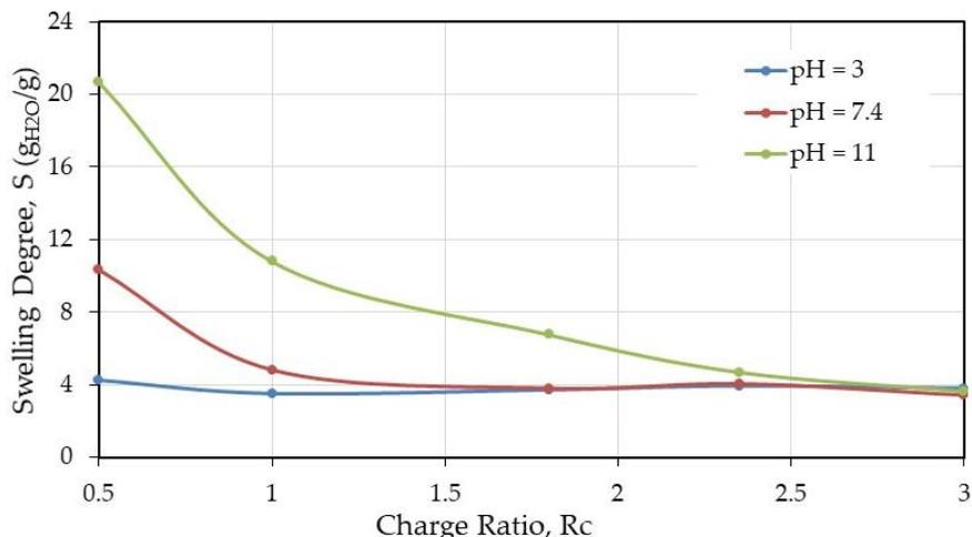
**Figure 4.** Swelling degree (g water/g dried material) as a function of the charge ratio after thermal treatment.
