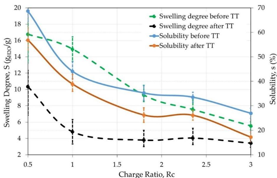
**Figure 3.** Influence of the thermal treatment (4 h at 120 °C) on PEC films solubility and degree of swelling as a function of charge ratio at pH = 7.4. Average values shown after repeating the experiment 4 times.
