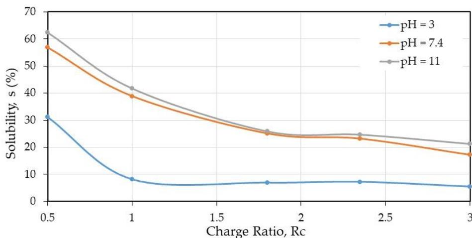
**Figure 5.** Partial solubility (%) at different pH on PEC films prepared in W/FA 50/50 *v/v* as a function of charge ratio.
