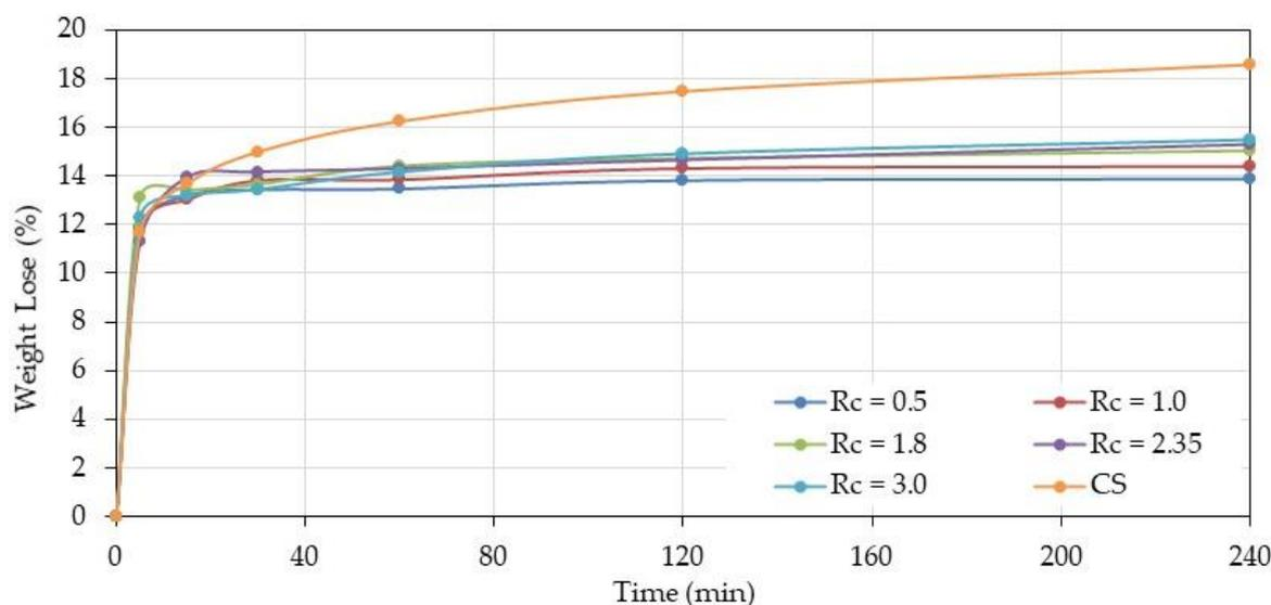
**Figure 1.** Weight loss of polyelectrolyte complex (PEC) at different chitosan (CS)/hyaluronan (HA) charge ratios  $R_c$  compared with pure chitosan (CS) prepared in water (W)/formic acid (FA) (50/50  $v/v$ ) as a function of time at 120  $^{\circ}\text{C}$ .
