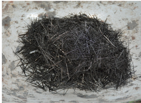
Fig. 3. Long straight steel fibers.
