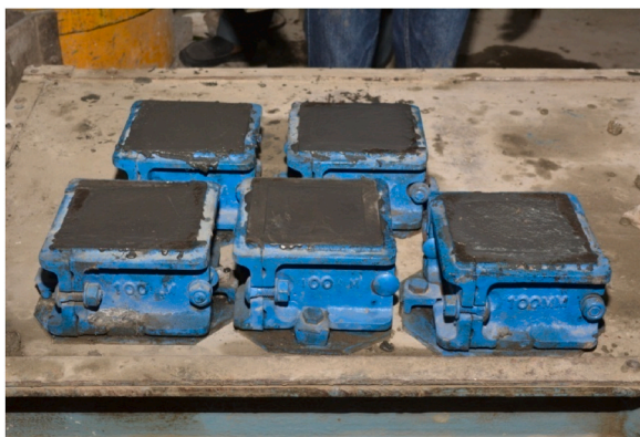
Fig. 6. Casting of UHPC specimens.
