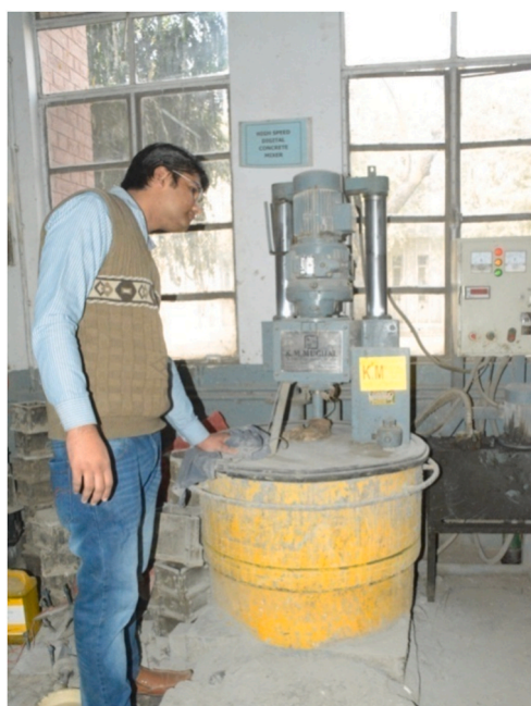
Fig. 5. Ordinary pan type mixer.
