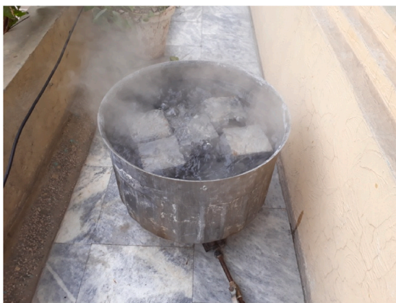
Fig. 7. Specimens under heat curing in a steel container.
