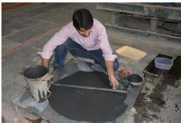
Fig. 8. Slump flow measurement of optimized mix.
