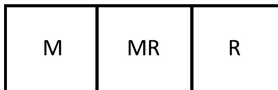
Figure 1. An example arrangement of three modules to make a larger intensified unit. Here a membrane separator (M), a membrane reactor (MR), and a reactor (R) are combined.
