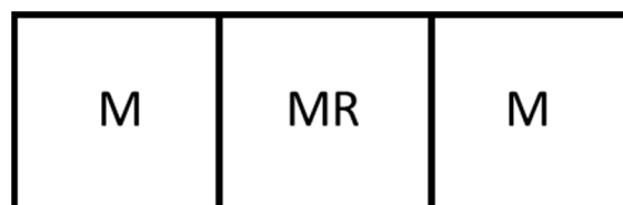
Figure 12. The optimum 3-mod design that maximizes the size of the AOS. In this case, this design can achieve a 67% larger space than the base case membrane reactor.
