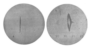
**Figure 1.** Pattern created by a ray of silver atoms in the original Stern–Gerlach experiment: **left**: without, **right**: with magnetic field.
