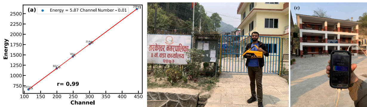
Fig. 2. (a) Energy calibration graph shows relation between energy and channel number. (b) At study area with Portable Gamma spectrometer Information System (PGIS 2) having specifications: NaI(Tl) crystal: 3"×3" (0.347 L), 512 channel spectrometer, energy range 20 keV - 3 MeV. (c) Mobile set connected via Bluetooth to the detector.
