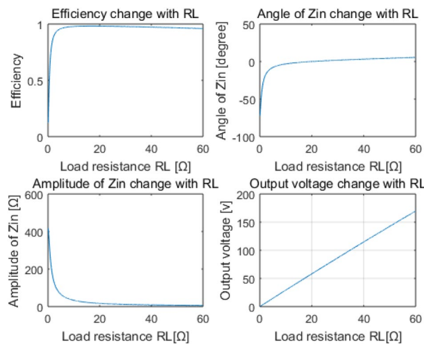
Figure 10. Main output characteristics of the proposed system working in COC mode, derived from MATLAB. (Created by “matlab R2016a” url: https://ww2.mathworks.cn/products/matlab.html ).
