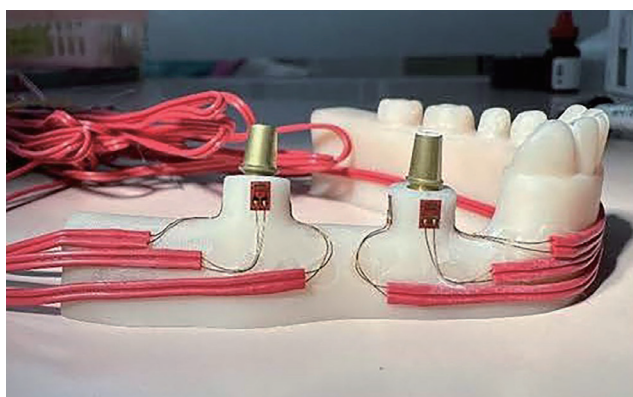
Fig. 4. Location of strain gauges on the model.
