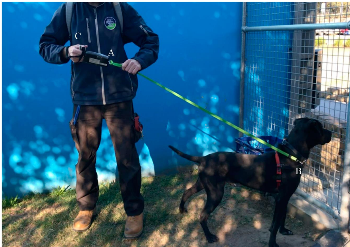
Figure 1. Demonstration of the canine leash tension meter. A 1.4-metre-long leash was connected to the tension meter (A) and then was attached to the collar and harness in front of the dog's chest (B). The handler held the metal handle on the other end of the tension meter (C).
