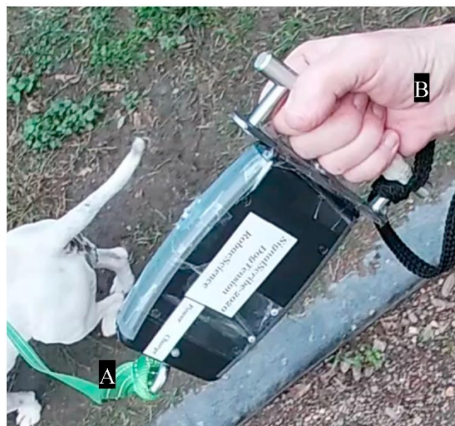
Figure 2. Close-up view of the canine leash tension meter. A 1.4-metre-long leash was connected to the tension meter through the stainless-steel eyebolt (A) and the handler held the metal handle on the other end of the tension meter (B).
