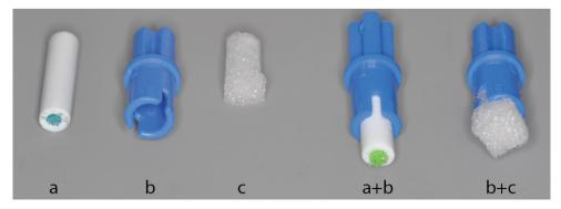
**Figure 3.** Two options for the modification to the connector pegs (**b**) to allow for insertion of the specimen pin: a 3 mm diameter tube with 0.1 mm nylon fibers (**a+b**); or a small plastazote plug (**b+c**).
