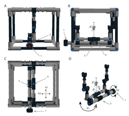
**Figure 2.** The IMp model shown from a side view (**A**), front view (**B**), top view (**C**) and without the stabilizing case exposing the pivot arm wherein the specimen is placed (**D**). Figure labels and abbreviations: pivot handle (**1**), 8 tooth gear (**2**), worm gear (**3**), connector peg that holds and rotates the specimen (**4**), axis of movement 1 (**A1**), axis of movement 2 (**A2**), axis of rotation 1 (**R1**) and axis of rotation 2 (**R2**).
