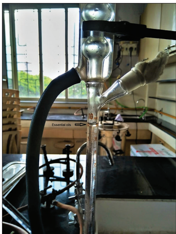
Figure 1: Collection of essential oils by Clevenger Apparatus
