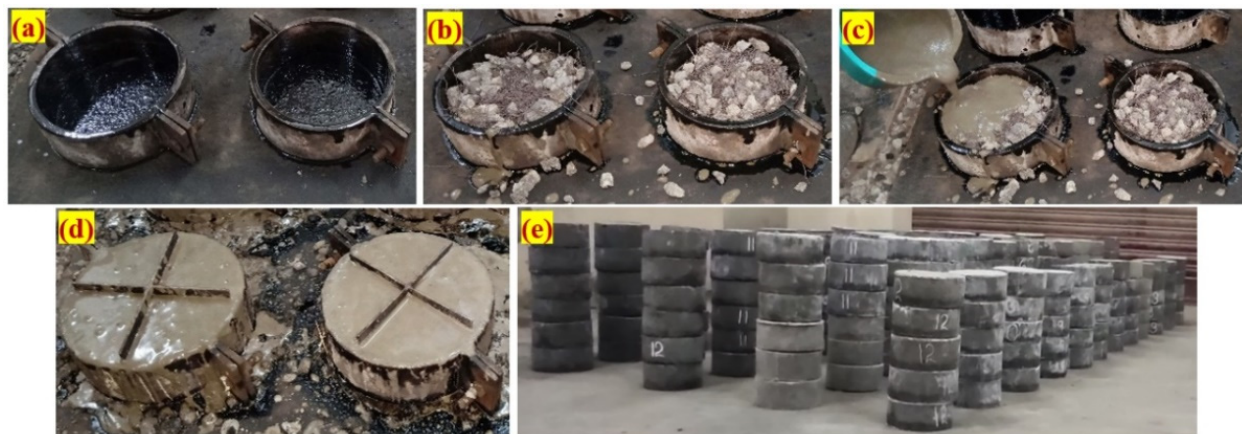
Figure 5. The fabrication method: (a) empty cylindrical mold; (b) fibres and coarse aggregate filled into the mold; (c) pouring of grout; (d) casted specimens with notch plate insertion; and (e) appearance of specimens, which were kept on the floor after demolding.
