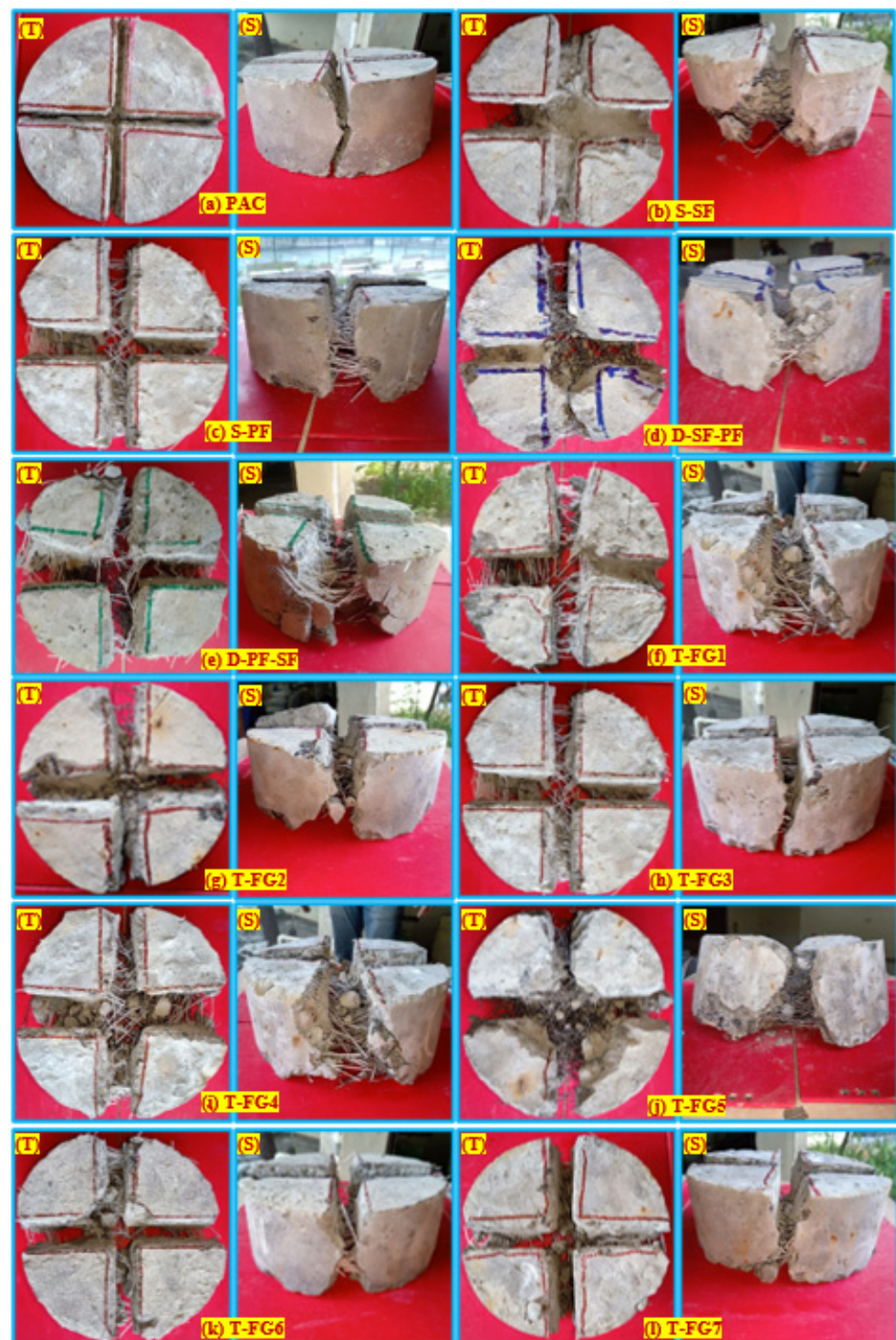
Figure 12. The failure pattern of the specimens under impact loading (a) PAC (b) S-SF (c) S-PF (d) D-SF-PF (e) D-PF-SF (f) T-FG1 (g) T-FG2 (h) T-FG3 (i) T-FG4 (j) T-FG5 (k) T-FG6 (l) T-FG7.
