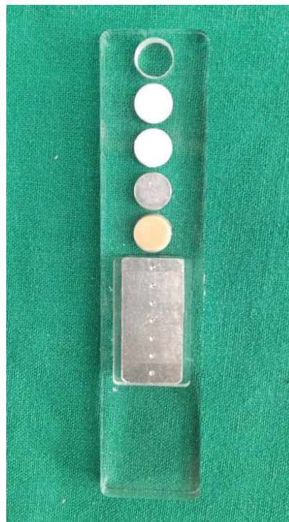
Fig. 1. The contrast phantom id composed of 2 parts. Five tissue-equivalent materials are contained in an acrylic block on the top. From the top, the materials are polymethylmethacrylate, polyoxymethylene, polytetrafluoroethylene, aluminum, and porcelain. The bottom contains an aluminum block with pits of various depths.
