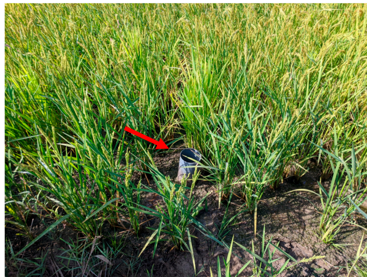
Figure 3. A water tube (red arrow) installed in a rice plot, during a dry period of AWD.
