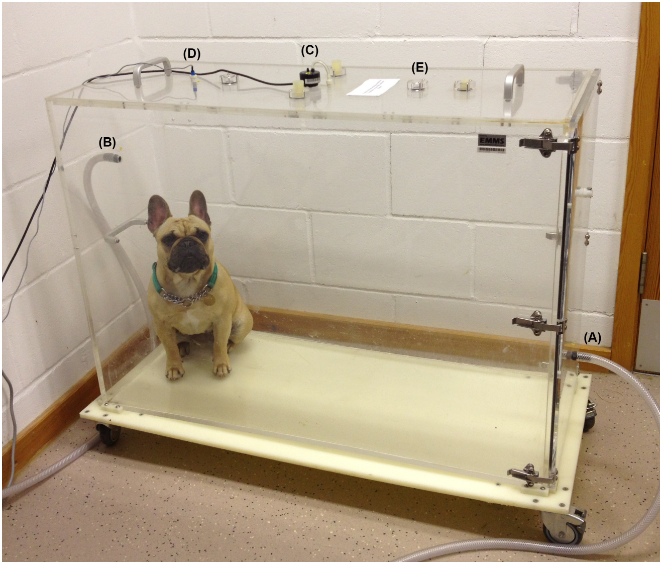
Fig 1. The chamber used for whole-body barometric plethysmography (WBBP) with a French bulldog undergoing the test. A pole of the chamber pressure differential transducer is opened to the top of the chamber (C); two inlets (A and B) are connected to the front and back of the chamber in order to ventilate with a bias flow of room air (20 L/minute); an audio sensor is located on the top of the chamber (D); together with pneumotachograph screens (E).
