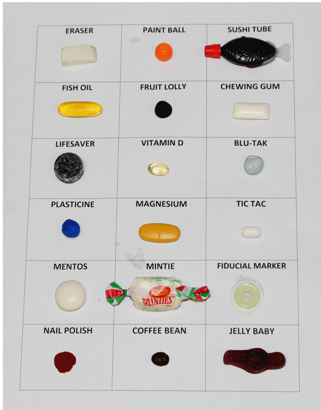
Figure 1 18 items investigated as surrogates for the commercially available fiducial markers—eraser, paint ball, sushi tube, fish oil capsule, fruit lolly, chewing gum, lifesaver, vitamin D, blu-tak, plasticine, magnesium tabsule, tic tac, mentos, mintie, commercial fiducial marker (IZI Multi-Modality, LifeHealthCare, Australia, included as a benchmark), nail polish, coffee bean, jelly baby sweet.
