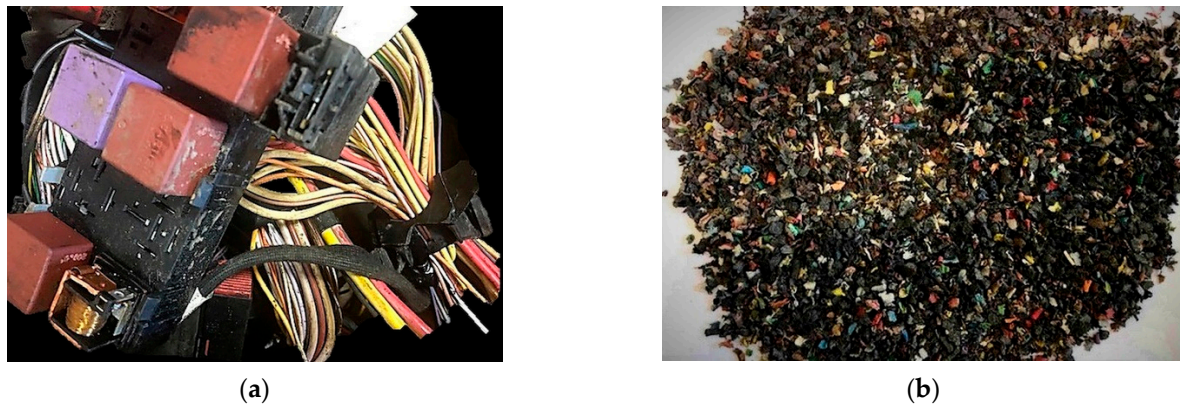
Figure 1. Origin wastes: (a) automotive originated cables wastes; (b) recovered and separated polymeric wastes of 1.8 mm fraction.
