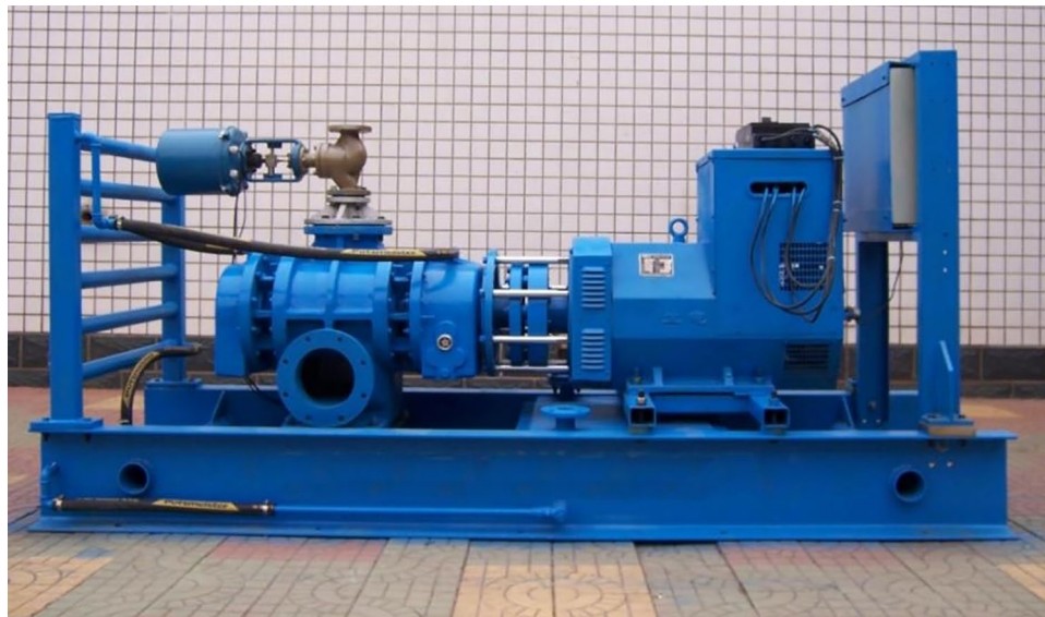
Figure 2. Low-quality waste heat recovery and utilization device with roots power machine as the core.
