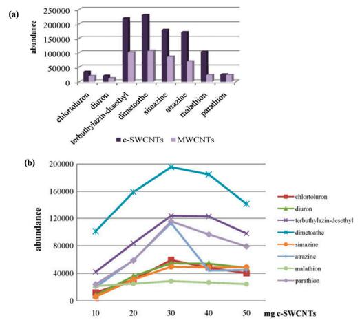
**Figure 7.** (a) Comparison of the performance of carboxylated (c)-SWCNTs and MWCNTs for the isolation of the selected pesticides from virgin olive oil samples. (b) Influence of the amount of c-SWCNTs packed in the solid-phase extraction (SPE) cartridge for the preconcentration of the selected pesticides from virgin olive oil samples [107].
