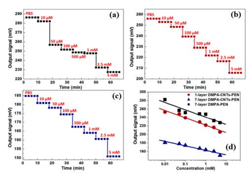
**Figure 5.** ConCap response curves toward penicillin G detection at different concentrations for LB film-incorporated EIS sensors: (a) seven-layer DMPA-penicillinase; (b) one-layer DMPA-CNTs-PEN; and (c) seven-layer DMPA-CNTs-PEN. (d) Calibration curve of ConCap responses for the LB films correlated with penicillin concentrations [93].
