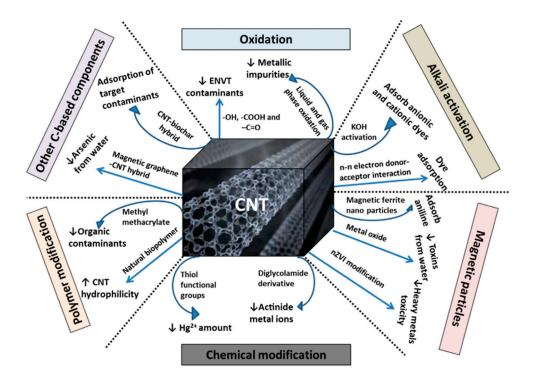
**Figure 8.** Schematic diagram representing different modification processes of CNTs for contaminant removal from water and wastewater (C: carbon; CNT: carbon nanotube; ENVT: environmental; Hg: mercury; KOH: potassium hydroxide) [129].
