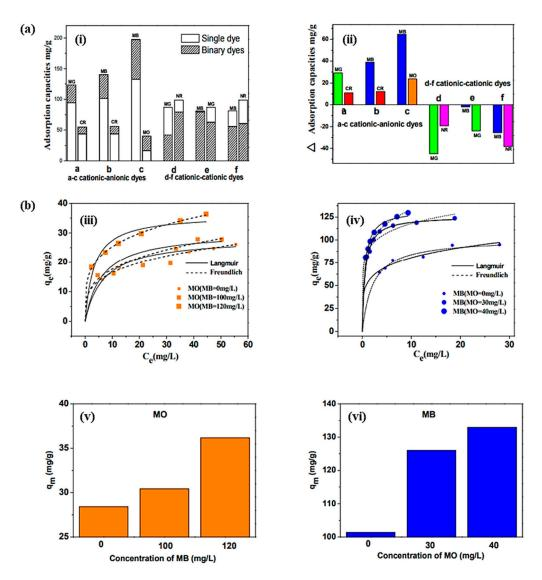
**Figure 9.** (a) (i) Adsorption capacities and (ii) their changes in single and binary dye systems. (b) Adsorption isotherms of methyl orange (MO) (iii) and methylene blue (MB) (iv) on CNTs/Fe@C fitted by the Langmuir and Freundlich models. The maximum adsorption capacity of MO (v) and MB (vi) increased with the concentration of the other dye [139].
