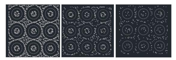
**Figure 10.** Hydrogen storage in nanotube bundles. Snapshots from grand canonical Monte Carlo simulations taken under 100 Bar pressure at 77 K (left), 175 K (middle), and 293 K (right) [173].
