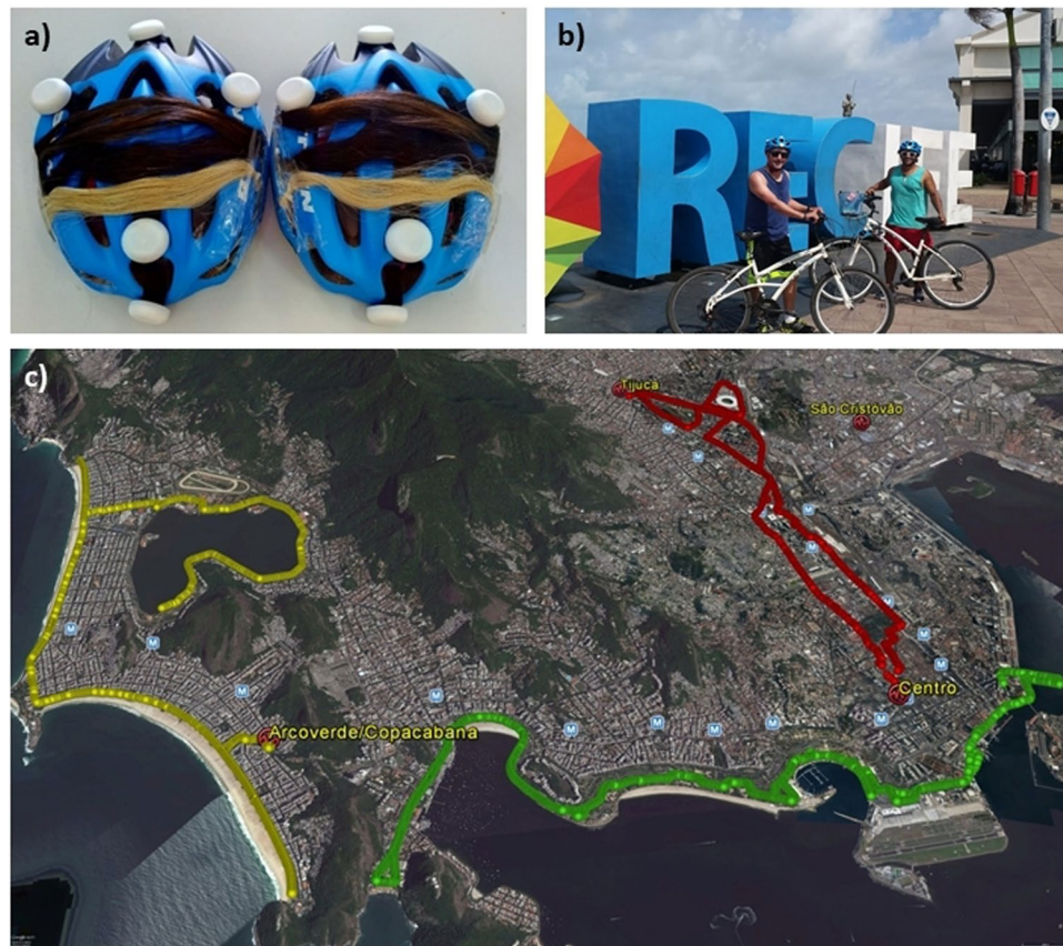
Figure 1. (a) Helmet with UV sensors and hair swatches (natural, colored, bleached/colored and gray). Fixed on the helmet. (b) Ordinary bikes adapted with scientific instruments. (c) Bike routes in Rio de Janeiro city in the experimental campaign of mobile measurement December 1 st –3 rd 2016 (red route – day 1, green route – day 2, yellow route – day 3) – Image: Google Earth Pro V 7.3.2.5776. Rio de Janeiro, Brazil. 22.9 S, 43.2 W, Eye alt 10.0 km. Data SIO, NOAA, U.S. Navy, NGA, GEBCO © 2018 Google.
