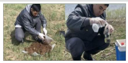
Fig. 1. Taking a water and soil sample for general chemical analysis.
