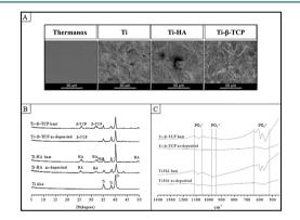
**Figure 1.** (A) SEM micrographs of Thermanox, grit-blasted Ti, Ti-HA, and Ti- $\beta$ -TCP surfaces. (B) X-ray diffraction spectra of grit-blasted Ti and as-deposited and heat treated Ti-HA and Ti- $\beta$ -TCP coatings. (C) Fourier transform infrared spectra of as-deposited and heat treated Ti-HA and Ti- $\beta$ -TCP.
