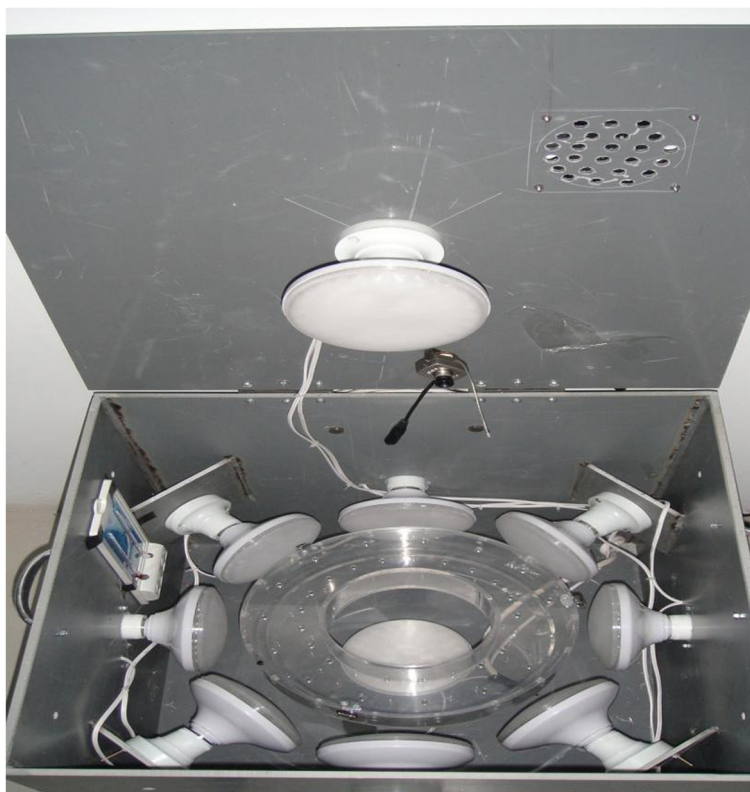
Figure 1 Annular illumination box for light-induced retinal damage in rats.
