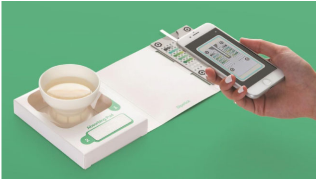
FIGURE 2: Digital smartphone urinalysis testing kit comprising a collection beaker, single urine dipstick and colour chart. The Dip.io urinalysis dipstick measures 10 different parameters (range of values in brackets): leukocytes (negative or 15/70/125/500 leukocytes/ \mu L), nitrates (negative or positive), glucose (negative or 100/250/500/1000 mg/dL), ketones (negative or 5/15/40/80 mg/dL), protein (negative or 15/30/100/300 mg/dL), blood (negative or 10/25/80/200 erythrocytes/ \mu L), pH (5.0, 5.5, 6.0, 6.5, 7.0, 7.5, 8.0, 8.5 or 9.0), urobilinogen (negative or 1/2/4/8 mg/dL), bilirubin (negative or 1/2/4 mg/dL) and specific gravity (1.000, 1.005, 1.010, 1.015, 1.020, 1.025 or 1.030). The dipstick result is analysed and processed via the smartphone camera using the company app (versions for Apple and Android are available). The results are then uploaded onto a secure portal and the overseeing clinician is notified of the new result. Currently one pack contains four tests, which can be reordered prior to the last test being used. Illustration courtesy of Health.io (Tel Aviv, Israel) reproduced with permission.
