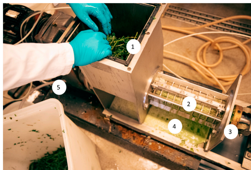
Figure 1. Pressing of alfalfa on Vincent CP-4 single-screw press. 1: Feeding with fresh alfalfa, 2: Screw and 0.5 mm filter matrix, 3: Discharge of pulp, 4: Discharge of the green juice, 5: Collection of the green juice. Photo: Flemming Leitorp.
