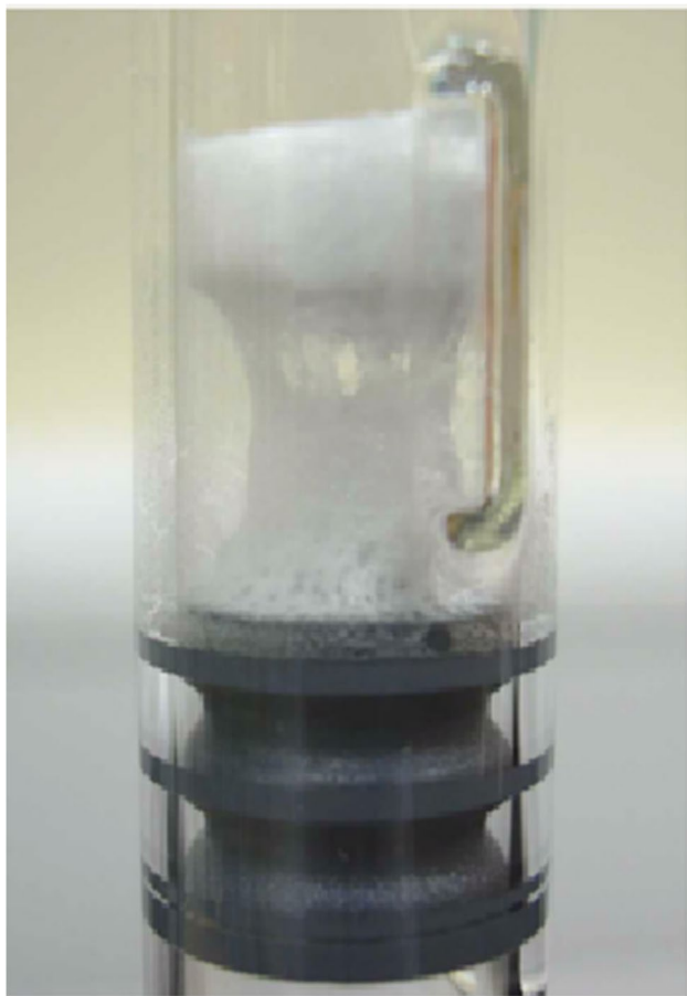
Fig. 6 A Sample of a Collapsed Cake occurring in DCCs
