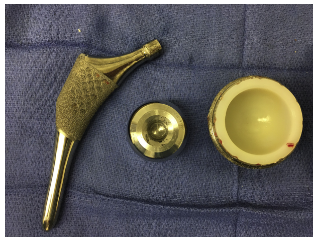
Figure 2. Explanted femoral stem, femoral head, and acetabular component. Damage to the trunnion is noted as well as metal residue.
