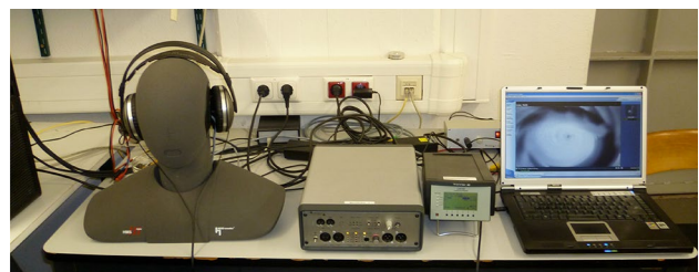
Fig. 1 Calibration system for Sennheiser earphones for white noise exposure
