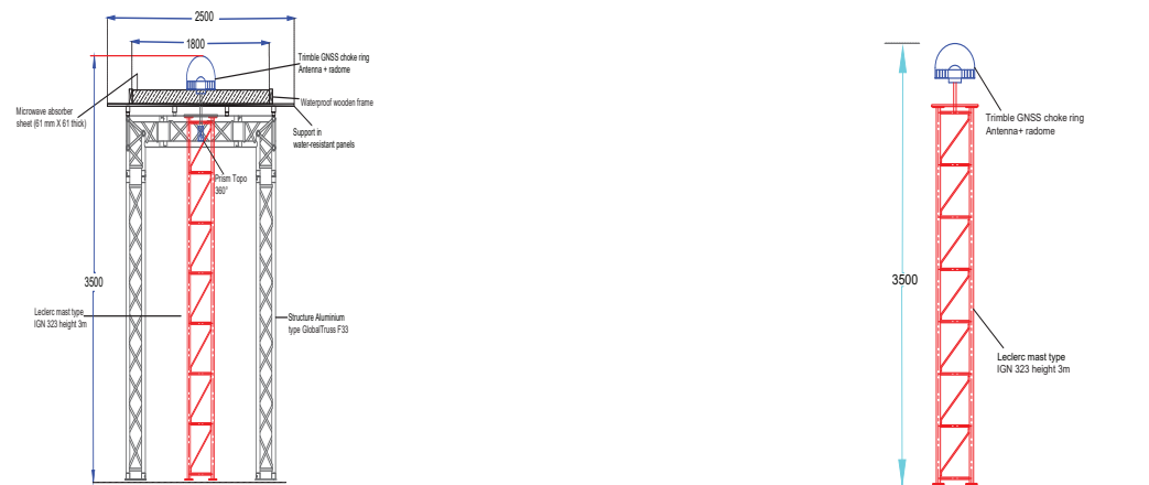
Figure 3. Autocad drawing of GNSS station KBG1 to the (left) and KBG2 to the (right). All the values are given in millimetres.
