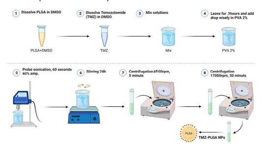
Figure 16. Preparation steps for the TMZ-PLGA-NPs using the emulsion solvent evaporation method.
