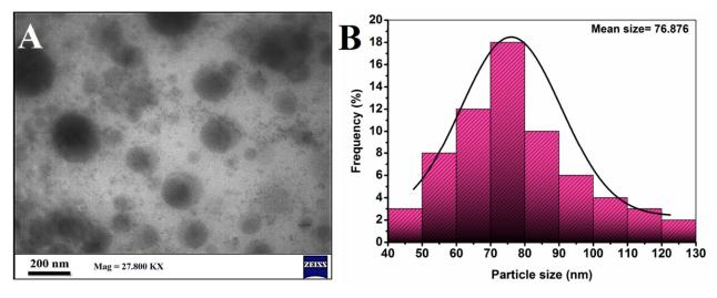
Figure 7. TEM images: (A) TMZ-PLGA-NPs; (B) particles size distributions.
