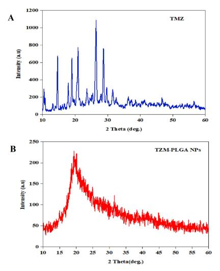
Figure 5. The XRD patterns: (A) free, pure TMZ in blue color; (B) TMZ-PLGA-NPs in red color.
