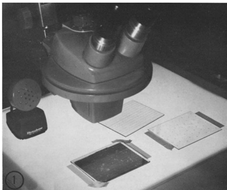
FIGURE 1 Arrangement used for quantitation of radioautographs. Negative micrographs were studied with a dissecting microscope. Also shown are the two types of template, one with guide lines for counting silver grains, the other with crosses for locating points to allow estimation of the relative area occupied by the various cell components in the same micrograph.
