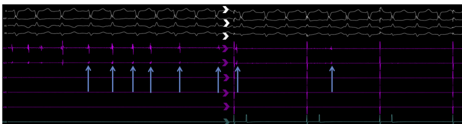
Figure 2 Right atrium–superior vena cava (SVC) potentials recorded at the ostium of the SVC with the Achieve mapping catheter (Medtronic Inc, Minneapolis, MN). Progressive delaying and real-time isolation of the SVC signals is shown by the arrows. Pacing artefacts during pacing from the decapolar catheter are observed at the right side of the image (started from -20^{\circ} in order to monitor phrenic nerve function).
