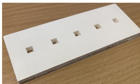
**Figure 1.** Photograph of the 3D-printed PMMA mold used to fabricate the implant specimens.
