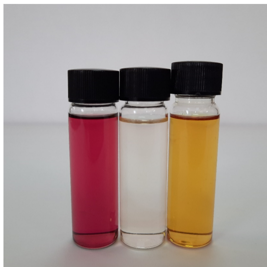
Fig. 1. Strong color change upon mixing iodine (far left; violet) with AZM (middle; colorless) to produce the AZM-I 2 CT complex (far right; brown) in the CH 2 Cl 2 solvent.
