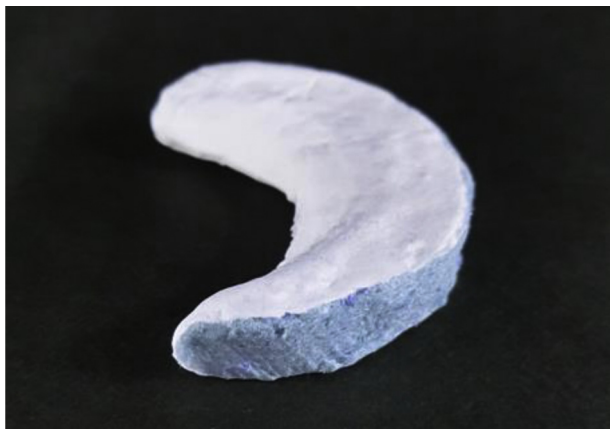
Fig 1. Meniscal scaffold composed of PGA coated with polylactic acid/caprolactone or P(LA/CL).
