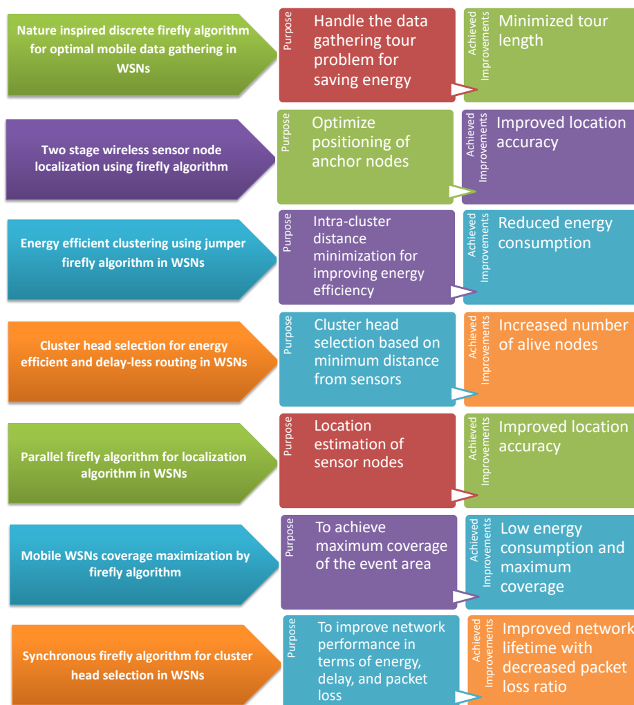
Figure 1. The impact of employing firefly algorithm in improving the performance of WSNs.
