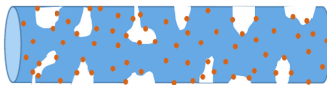
Figure 8. Schematic illustration of the distribution of Ag nanoparticles in \text{Ag@TiO}_2 nanofibers.
