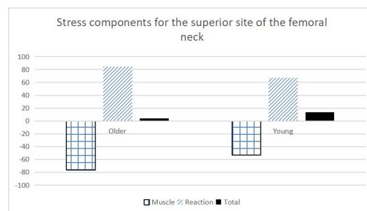
Fig 5. Components for the peak stress at the superior site of the femoral neck during stair ascent at peak 1. Stresses derived from muscle, reaction components and the total stress for each age group were shown.
