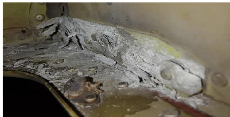
Figure 6. Corrosion on Wing Spar.
